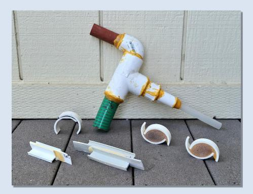
Applications: Bonding PVC liners and pipes with CIPP liners, concrete, and other substrates (i.e. steel, brick, wood, etc.)
